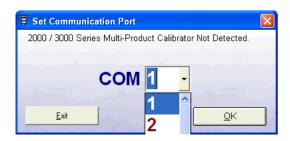
On starting the virtual front panel for the first time, a COM port selection screen will be displayed. Click on the COM port that is connected to your 3000 Series calibrator to continue.
